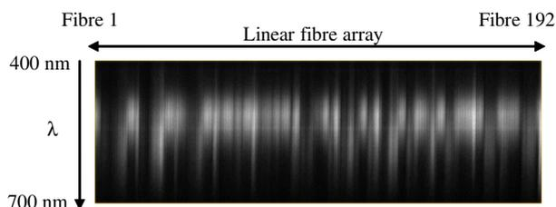
**Figure 3.** A typical spectrally dispersed image recorded on the foveal CCD.
