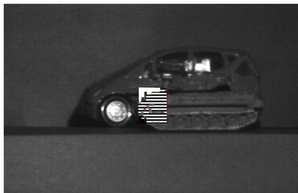
**Figure 5.** The image of the tank and car in the combined field of view. Pixels inside the fovea are assigned pure white or hatched to indicate similarity to training spectra for the car and tank respectively. Unclassified pixels retain greyscale values. This frame was taken from an animation that is available at [stacks.iop.org/JOptA/7/S298](http://stacks.iop.org/JOptA/7/S298).
