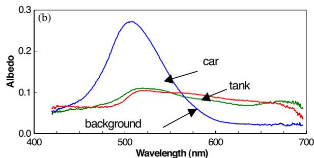
**Figure 4.** (a) A conventional, three-colour photograph of a scene consisting of a green model tank and a green model car against a background colour to be a close match to the colour of the tank and (b) the measured albedos of the three spectral classes.
