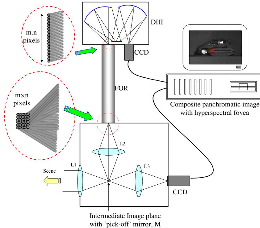
**Figure 1.** A schematic diagram of the instrument described. One camera is used to record a wide-field, panchromatic peripheral image, while another records a reformatted, spectrally dispersed image, which is used to form a hyperspectral fovea.
