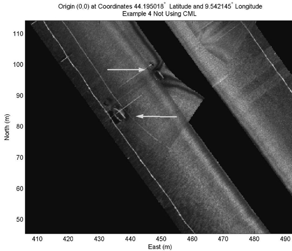
Fig. 23. Example 3: Not using CML. The Kalman-RTS strategy can be used to propagate the acoustic fix to points that occur in the trajectory before the fix.
