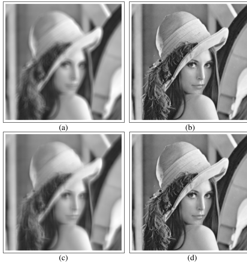
Fig. 5. Images with lens position at 2.5mm acquired with (a) no implementation of phase mask, with (b) mechanically compensation, -with (c) implementation of phase mask before restoration and (d) with implementation of phase mask after restoration.
